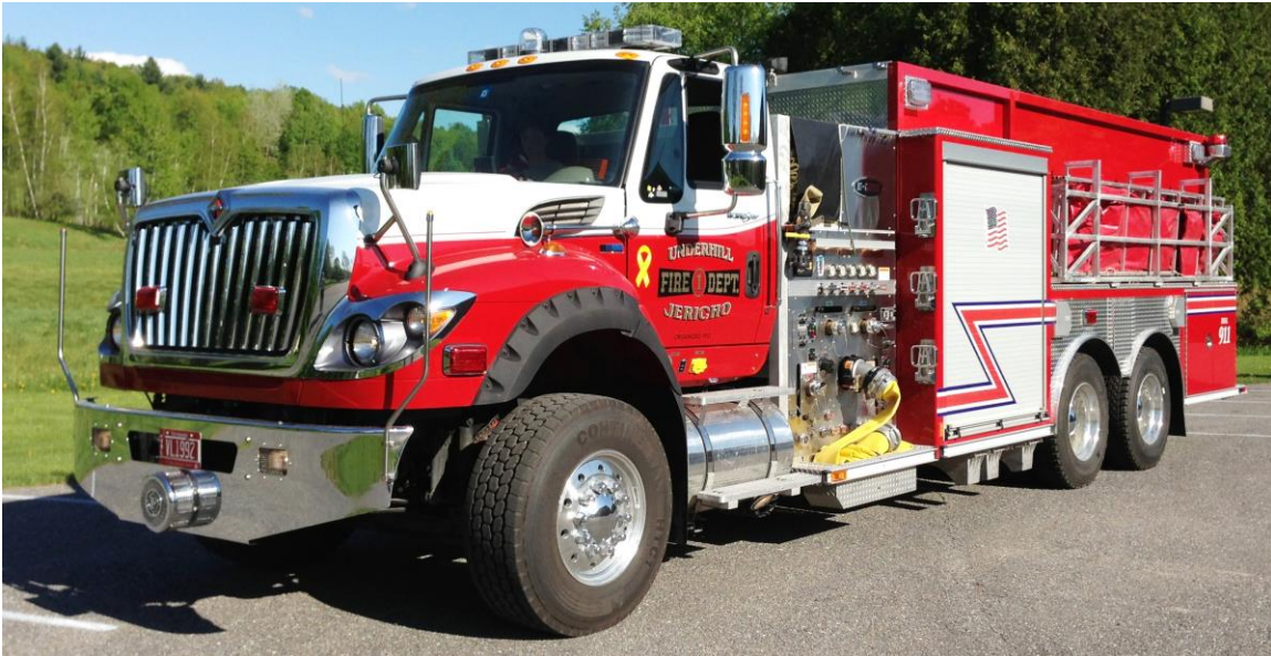
2013 International; 475 hp diesel; automatic transmission; tandem axle; 2650 gallons of water; 2500 gallon portable tank; 1250 GPM pump; and 2000 feet of 5 inch large diameter hose. Cost $350,000
