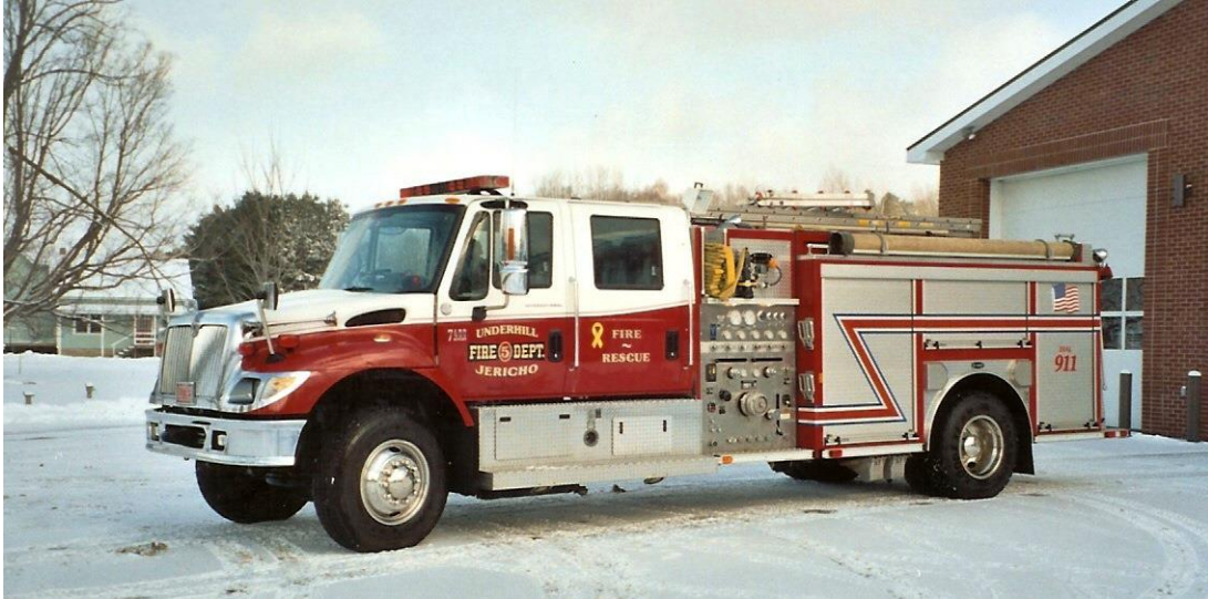
First 2002 International Crew Cab Model 7400 Built By Navistar International, truck has a 1250 GPM pump; carries 1000 feet of 5 inch hose and has an aluminum body manufactured by Emergency One.
