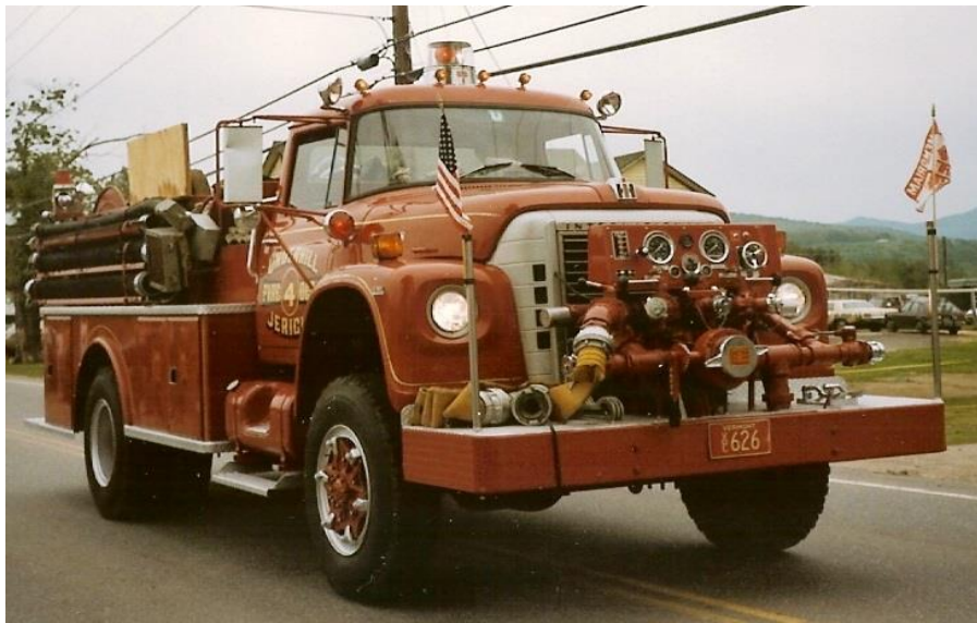
1977 International 4x4 with 1500 GPM pump and 2000 feet of 4 inch hose on a reel
