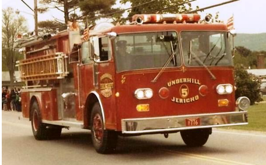
1982 Duplex Custom 5 man cab with an E-One Aluminum body and a 2000 GPM pump
