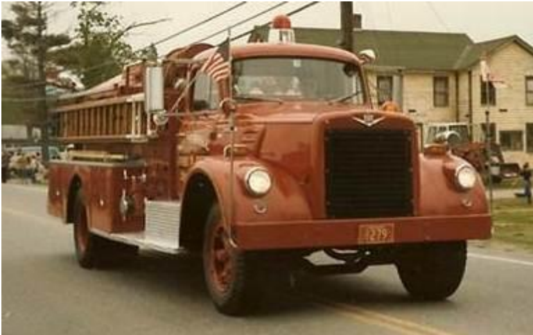
1963 International with a 750 GPM pump and 500 gallons of water
