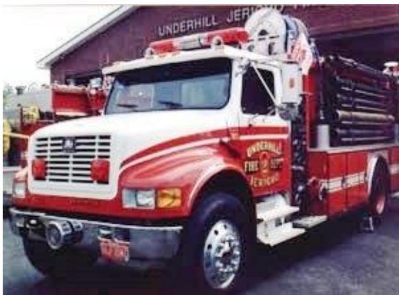
1990 International 1700 gallon tanker with 480 GPM pump and foam capabilities with aluminum body by American Eagle
