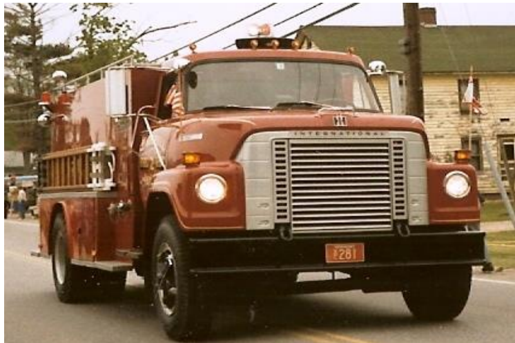
1970 International 2000 gallon tanker with 350 GPM pump
