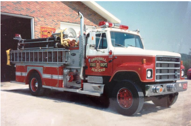
1985 International with 2000 GPM pump and E-One Aluminum Body
