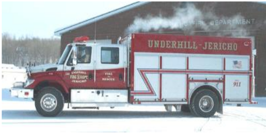
2002 International 5 Man Cab w/aluminum body; carries extrication equipment
