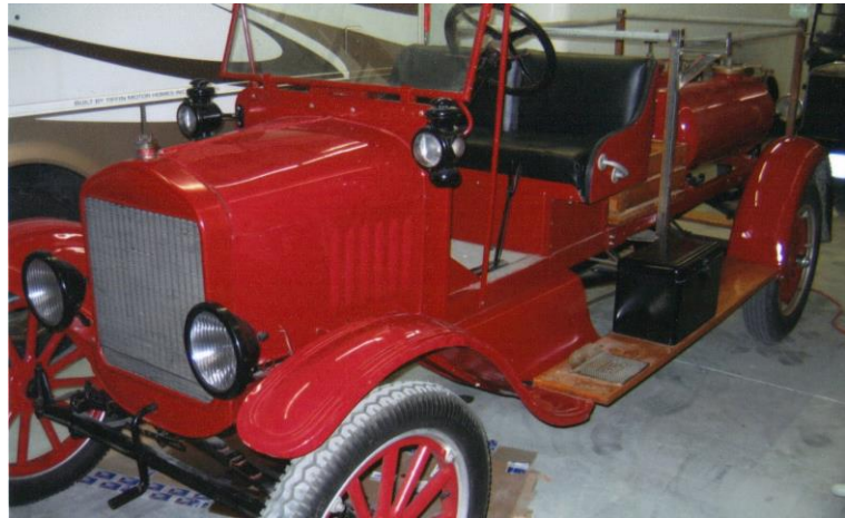
1923 Model TT Ford Fire Truck with two 40 gallon tanks
