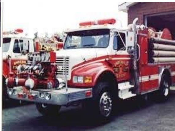
1990 International 1700 gallon tanker with 480 GPM pump and foam capabilities with aluminum body by American Eagle
